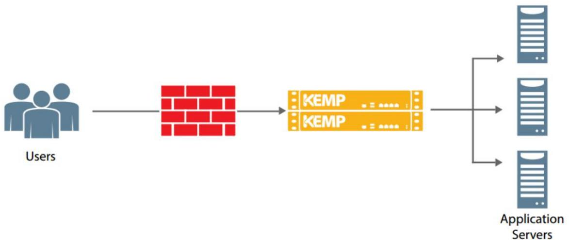
Figure 2-1: Typical LoadMaster topology
